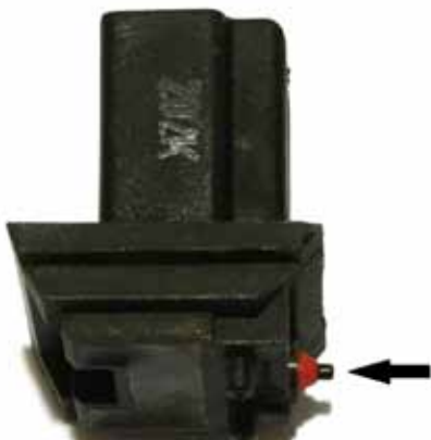
Microswitch from a 307 Tailgate Release. The arrow indicates the tiny button that is depressed when you press the release from the outside. To get an idea of size, the whole part pictured is about 30mm long.
