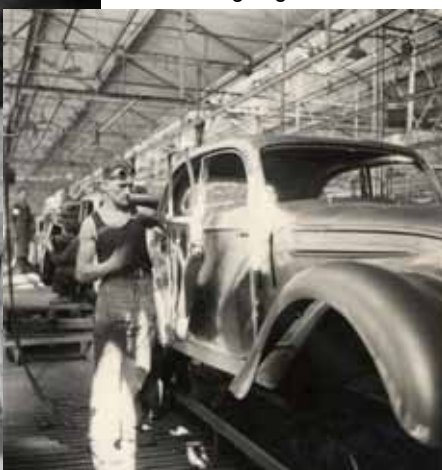
202 line: Fitting hinges on a rear door.
