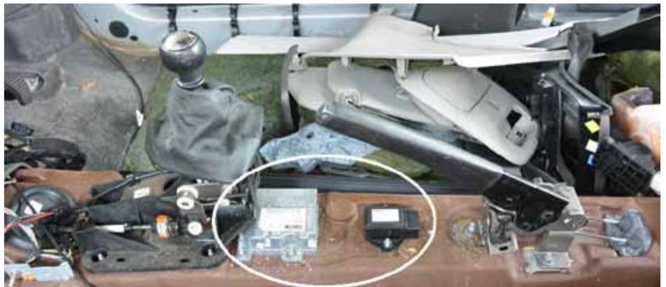
G-force sensors that trigger airbag deployment.
