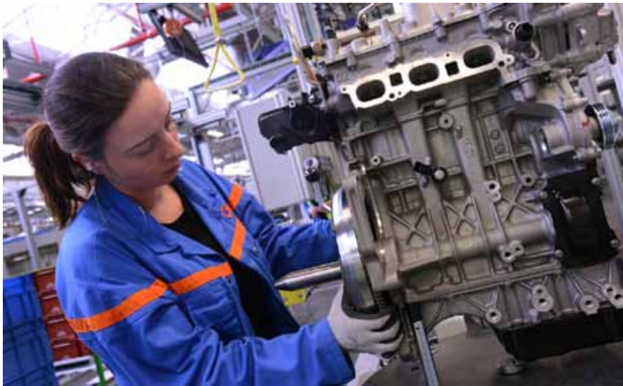
Emissions beater: A woman finishes off a PureTech 1.2-litre engine at the Douvrin factory.
