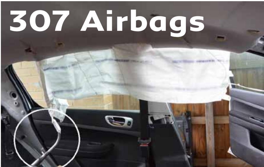
Photo #1 – Curtain airbag deployed - metal pipe with explosive charge circled.
